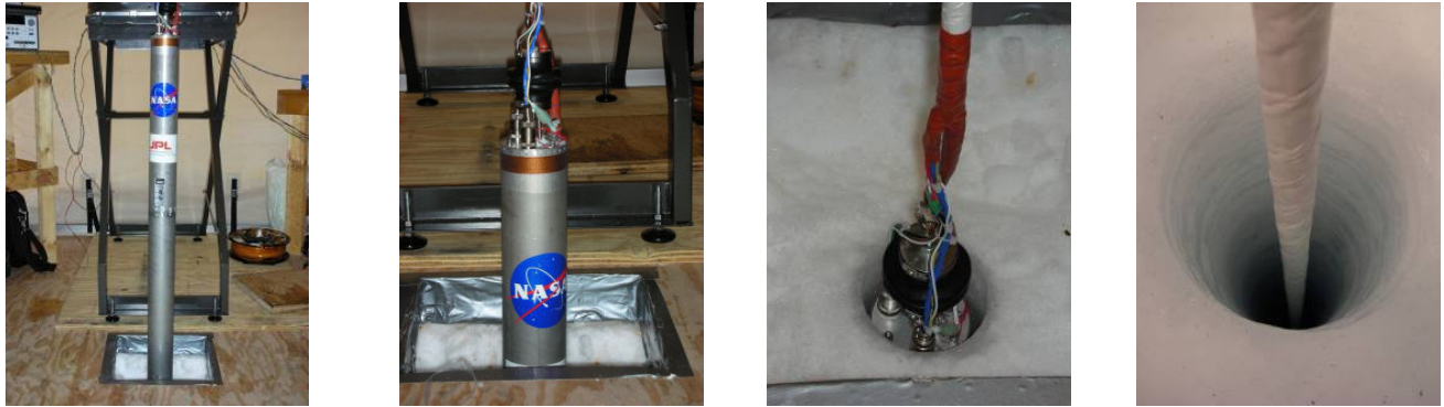
Figure 2: A 7 cm diameter thermal drill descends into the Greenland ice cap returning meltwater for analysis through an aerogel-insulated tether. In the final frame, the drill is 47 m below the surface (images from JPL).
