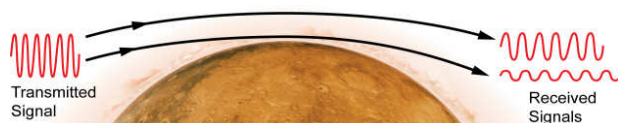
Fig. 1. Schematic of the change in the frequency and amplitude of sat-sat occultation signals.
