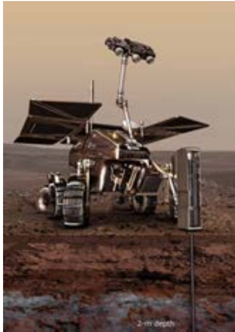
(Right) Figure 5.3. Artistic representation of the ExoMars Schiaparelli drill, deployed on Mars. This drill has a 1 cm diameter and is designed for up to 2 m depth, although in a rocky environment. (Image credit ESA).
