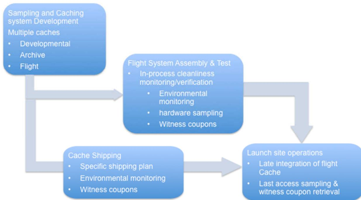
**Figure 24.** Notional parallel paths for sample system development and flight system development, with late integration into the flight system.
