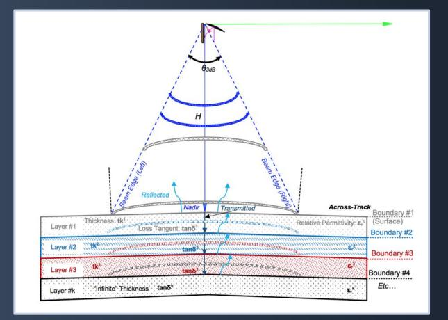
Ground-track spacing: 20 km at the equator Vertical resolution: 1 m in free space Along-track resolution: 30 m Across-track footprint: 1.5 km Modes: single track and repeat track
