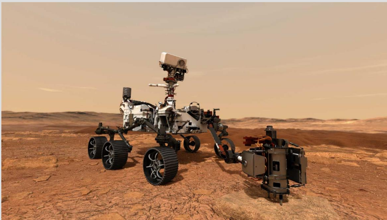
Artist's concept of NASA's Mars 2020 rover using its drill to core a rock sample on Mars
