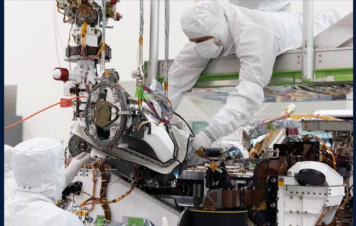
The bit carousel for the Mars 2020 mission is attached to the front end of the rover, August 5, 2019. Image Credit: NASA/JPL-Caltech
