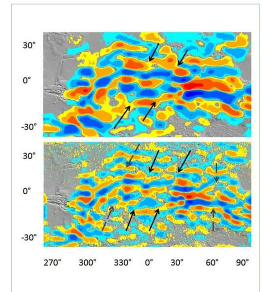
**Fig.3** A map of the crustal magnetic fields near Meridiana Planum using (top) 400 km MGS data and (bottom) downward continued, de-noised MGS data. Putative transform faults (black arrows) are more evident in the enhanced dataset. Gradiometry from multiple spacecraft would offer even more enhanced maps.
