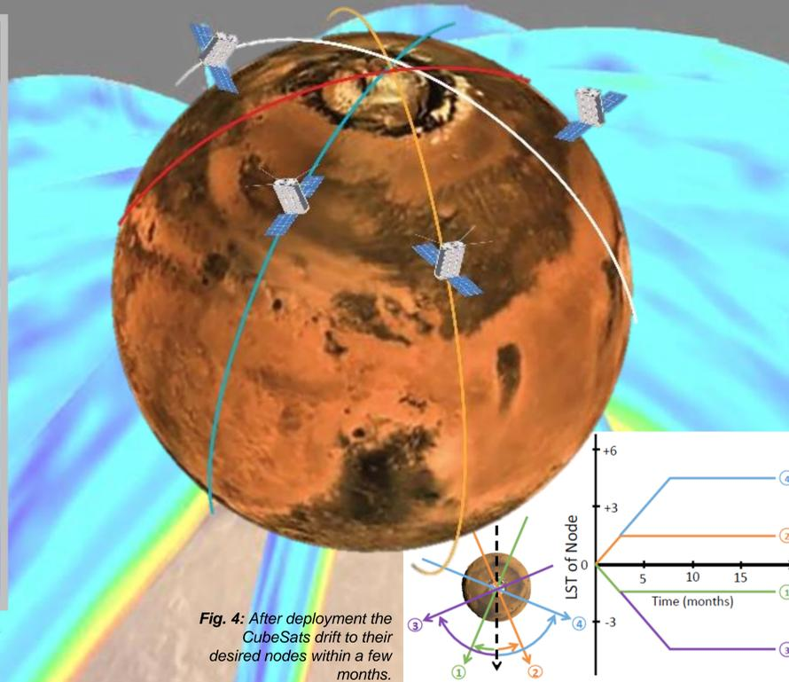
Fig. 4: After deployment the CubeSats drift to their desired nodes within a few months.
