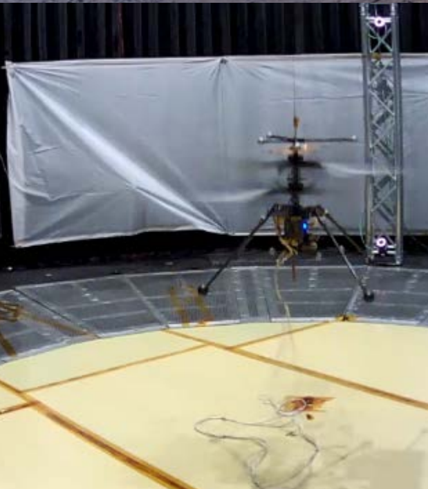
Full-scale free flight testing in JPL Space Simulator
