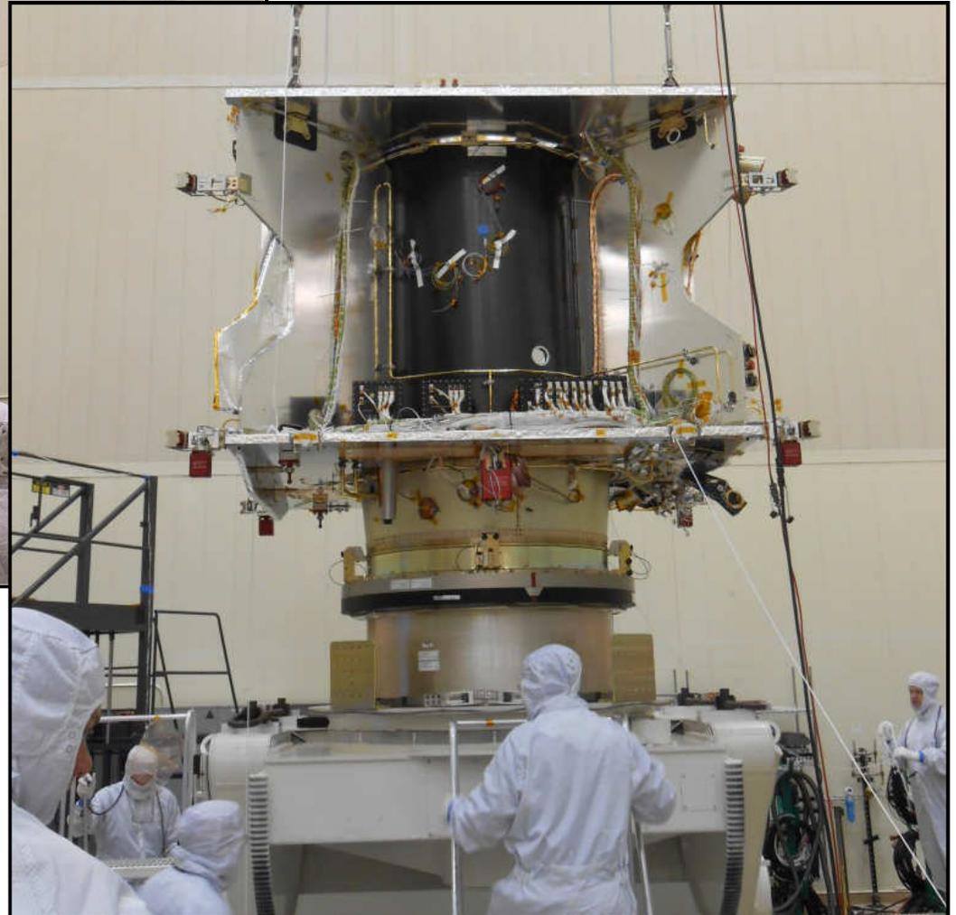
*Recent lift onto rotation fixture, showing current ATLO configuration*
