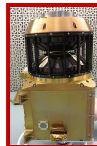
*Solar Wind Ion Analyzer; Jasper Halekas, SSL*
