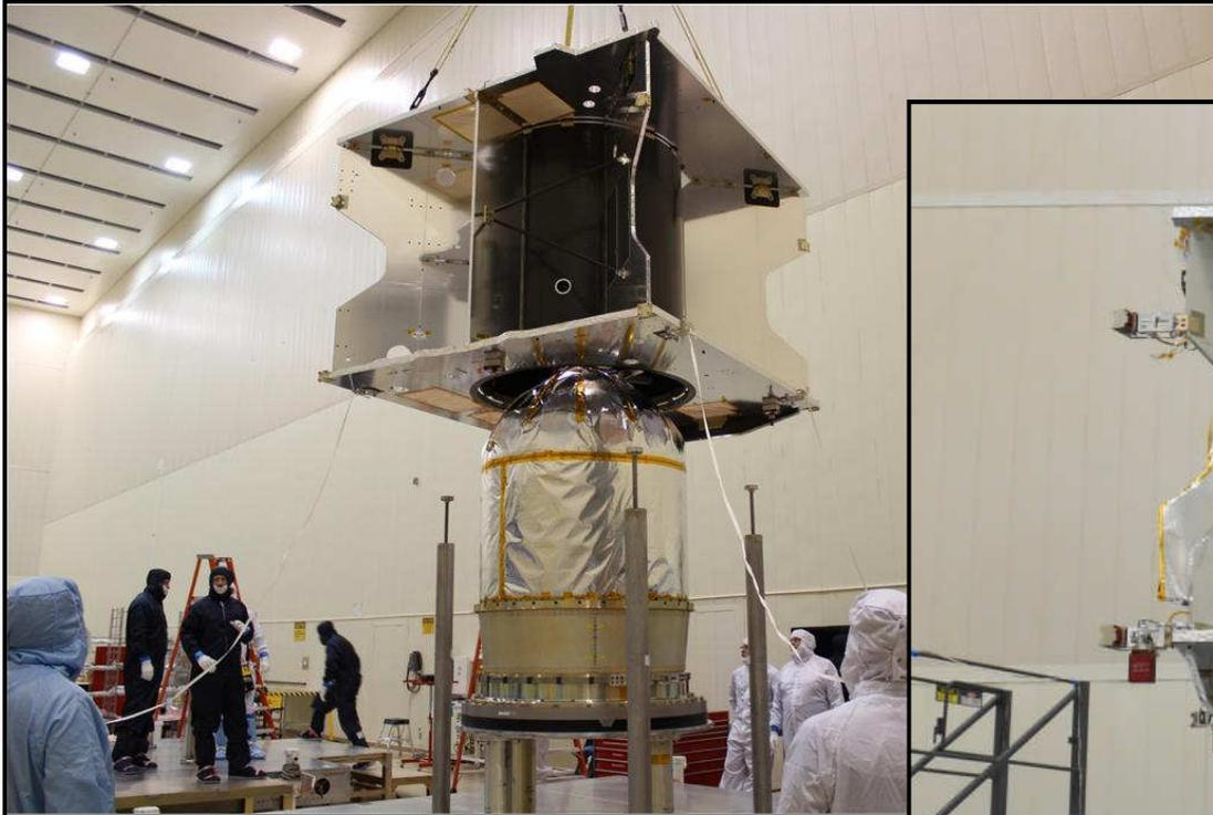
*Integration of core structure with fuel tank*
