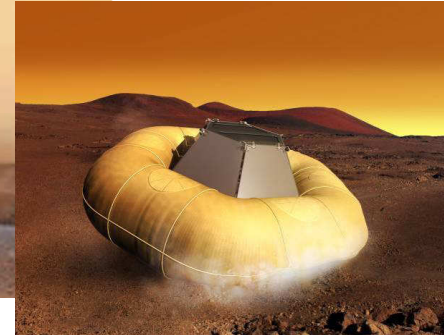
Descent and landing GNC, Airbags, throttleable retro-rockets
