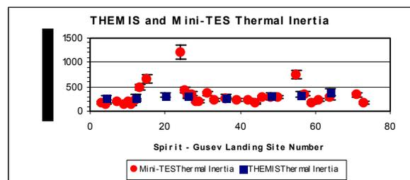
**Figure 2.** Plot comparing the thermal inertia trends between THEMIS-derived thermal inertia from orbit and Mini-TES-derived thermal inertia of the surface at the MER-Spirit landing site.
