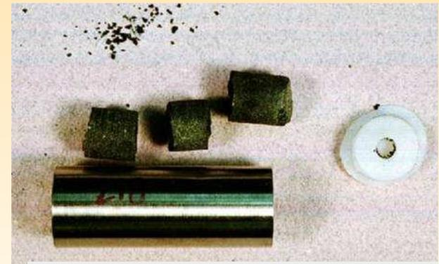
Test sample that experienced 3400 g in a tube that remained sealed—such a sample would meet ND-SAG requirements
